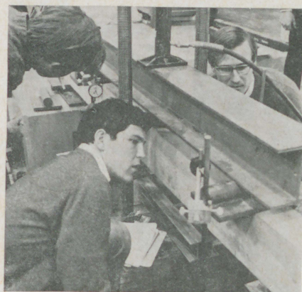
Architecture graduate students testing structural concrete beams at Engineering Laboratory in Engineering Quadrangle and acquiring "basic knowledge of specific facts which the architect must possess."
